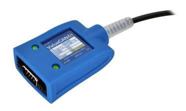
Real Time Acceleration and Standalone Mode Enable High Speed Flashing, Gateway, and ECU simulation The ValueCAN 4-1 FD can load real-time Function Block scripts and C code created with Vehicle Spy Professional, which execute in real time at microsecond resolution. Scripts can be controlled and monitored with a PC or operate standalone.
