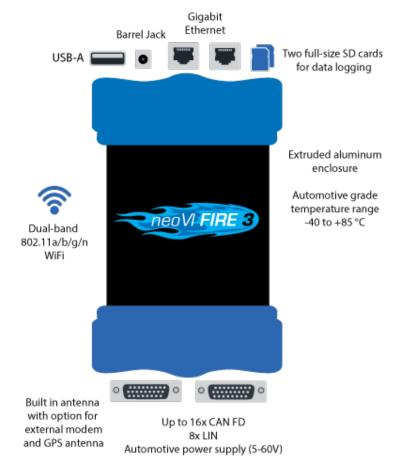
The neoVI Fire 3 also has a real-time clock for hardware timestamping of all messages. A robust power management system automatically powers down the neoVI Fire 3 and it wakes up again based on network activity or the connection of a PC.
